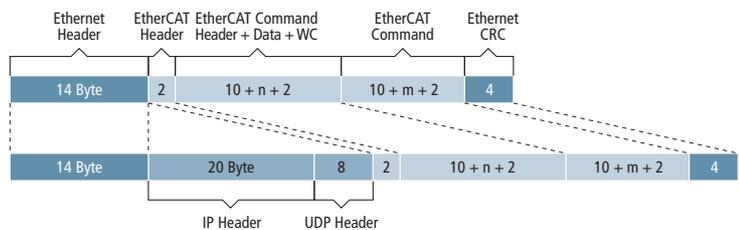
EtherCAT telegram structure (with and without UDP)
